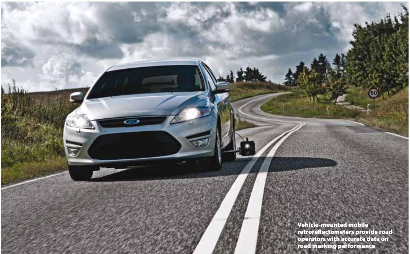
Vehicle-mounted mobile retroreflectometers provide road operators with accurate data on road marking performance
