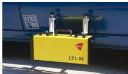
The system also offers the opportunity to accurately measure both white and yellow markings automatically without requiring recalibration. Other key features include good linearity up to at least 2,000 mcd/lx/m<sup>2</sup>; measurement of profiled markings up to 25mm; easy, once-daily field calibration traceable to national standards; and the suppression of daylight to retain measurement accuracy.
