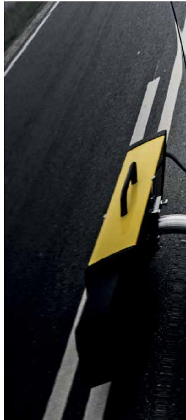
of  $\pm 5\%$ , during all driving conditions. Because of its ability to automatically compensate for movements, the LTL-M can be mounted on almost any type of vehicle and can be transferred between vehicles easily. LTL-M is almost as simple to operate as a handheld device.
