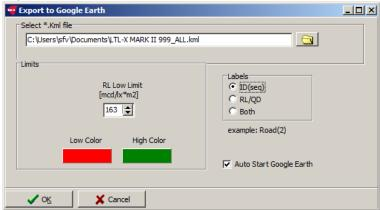
If log data represents downloaded data (not data from a protected file) the file name will be a combination of the instrument type, the serial number (e.g. 428) and the selected Series ID. The extension must be .kml.
