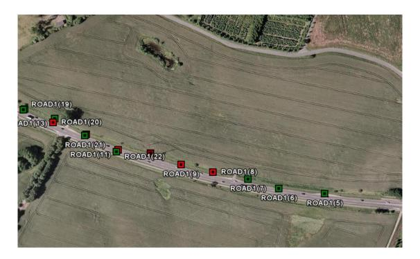
The text shown with the data point in GE is the Series ID and sequence number for the  $R_L$  measurements. If you click on a data point in GE a box will pop up showing the further information about the measurement e.g. the  $R_L$  value.
