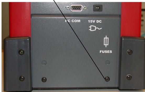
Loosen the big screw at the battery cover. You can now remove the cover.
