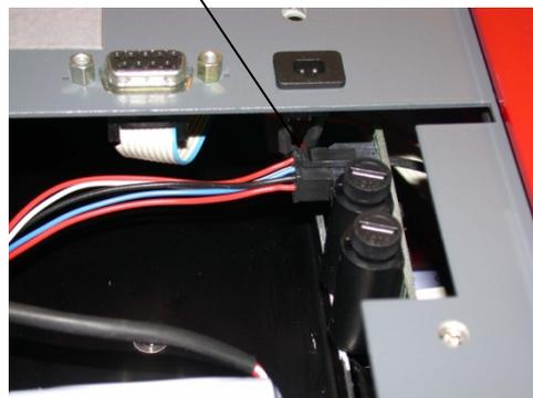
The battery can now be removed and replaced. Refit in reverse order. Please check your local regulations for disposal of the battery.
