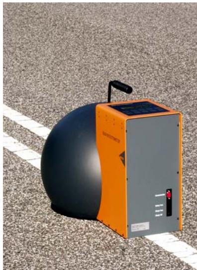
The sphere illumination varies due to the relative large observation port. This variation, caused by the road influence, is compensated by a light meter cell near the port. The light meter cell is connected to the detector circuit by an optical fiber. The ratio between observer and sphere illumination is a direct measure for the Qd value.
