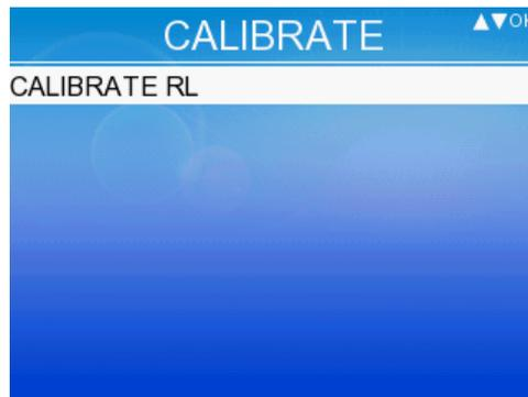
Check the value displayed and, if necessary, adjust it using the DOWN or UP buttons so it match the value stamped on the calibration unit.
