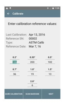
• Calibrate the GRX: Press 'Dark calibration' and follow the instruction on the screen (i.e. point the instrument in a direction with nothing 10 m/33 feet in front of it and away from any light source).
