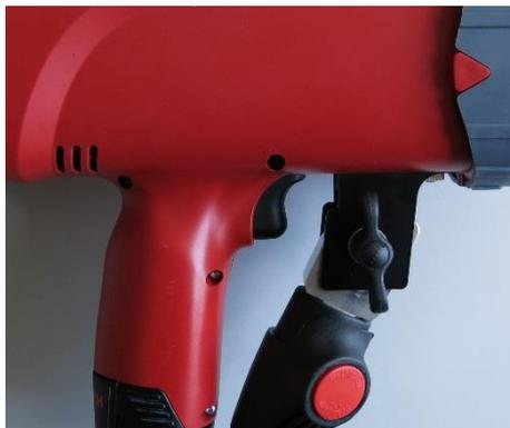
**Note:** In order to obtain correct readings when taking measurements with the extension pole, make sure that the GRX angle adapter plate is in full contact with the sign surface.
