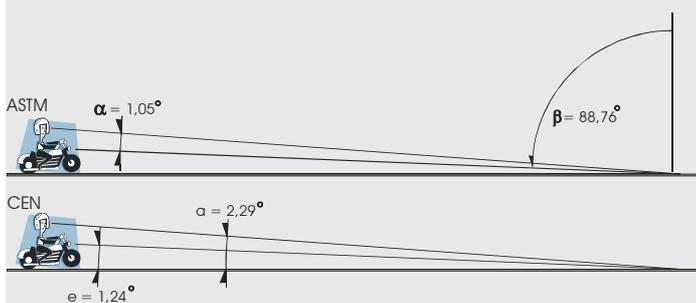
Figure 5: Angles defining the '30 m geometry' in ASTM and CEN standards.
