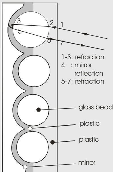
Figure 6: A glass beaded sheeting of the enclosed lens type.
