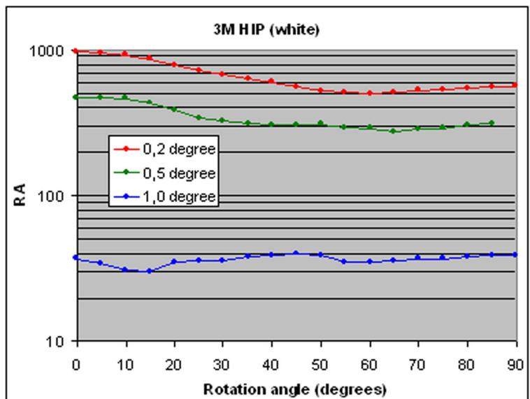
**Figure 7:**  $R_A$  values measured with a RetroSign GR3 ASTM on 3M DG3 material.
