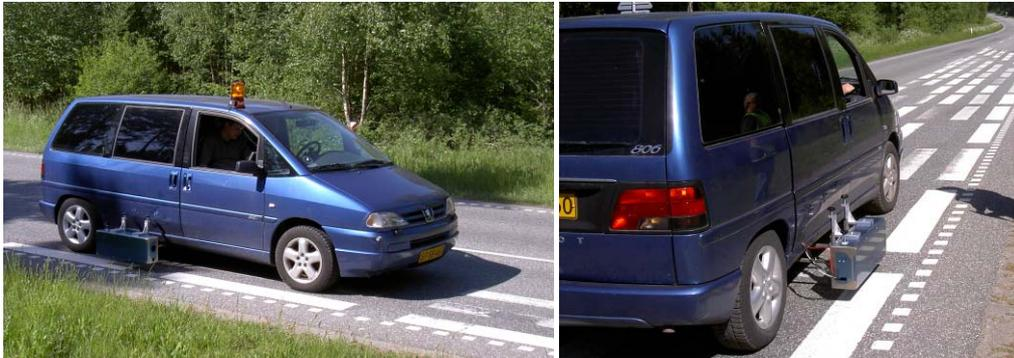
*Figure 1 The LTL-M mounted on a Peugeot van.*
